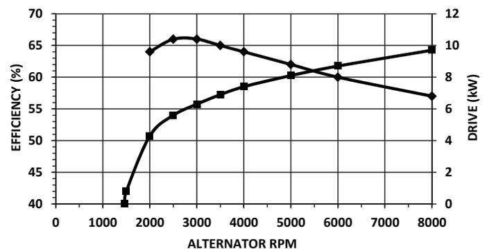
The measurements listed on the curves are taken at the listed ambient temperatures with a stabilized machine temperature, as per SAE J56. The shaded area highlights output available at typical engine idle alternator speed.
